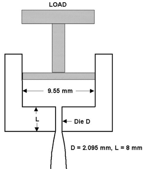
Fig. 2-3 Schematic of a melt indexer. ASTM D-1238 Under the conditions of the melt index measurement with the 2.16 kg load, the wall shear stress can be calculated to be  $\tau_w = 1.94 \times 10^4$  Pa (=2.814 psi) and the wall shear rate approximately  $\dot{\gamma} = (1838/\rho)$  MI where  $\rho$  is the melt density. Assuming  $\rho = 766$  kg/m<sup>3</sup> for a typical PE melt at 190°C, we get  $\dot{\gamma} = 2.4 \times$  MI.
