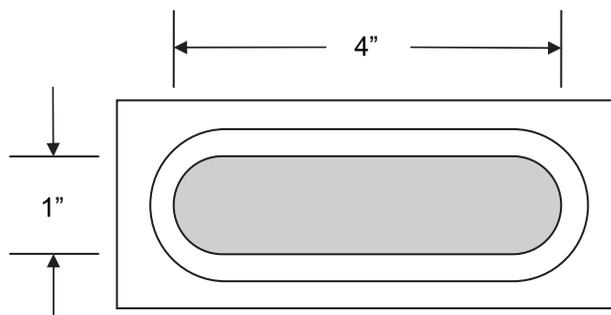
**Fig. 6-18** Racetrack exit from feed block to match die entrance with rounded corners to prevent degradation.
