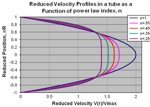
**Fig. 6-16** Plot of reduced velocity profiles for flow in a tube as a function of the power law index,  $n$  showing the blunt flow (plug flow) front increasing as  $n$  decreases.
