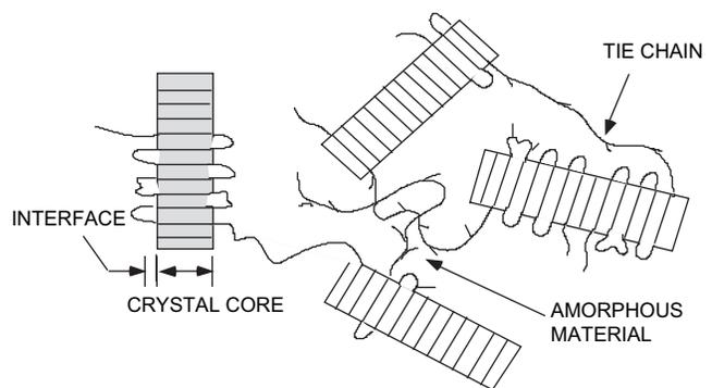
Fig. 2-8 Crystalline and amorphous regions of a semicrystalline polymer.
