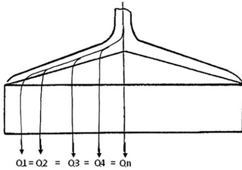
**Fig. 6-13** Desired uniform volumetric flow rate ( $Q$ ) across width of die.
