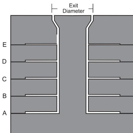
**Fig. 7-4** Stacked type of coextrusion die.
