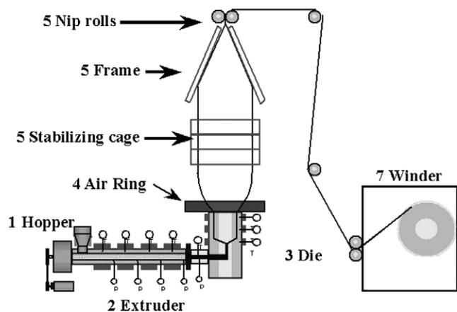
Fig. 9-1 Blown film process.
