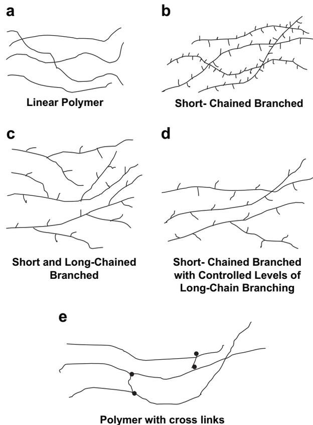
**Fig. 2-10** Schematic of common polymer chain structures. (a) Linear polymer; (b) short-chained branched; (c) short- and long-chained branched; (d) short-chained branched with controlled levels of long-chain branching; (e) polymer with cross links.
