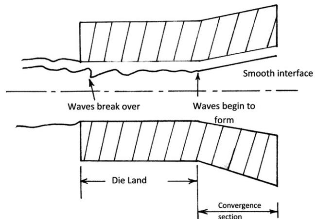
**Fig. 6-31** Onset of ‘zig-zag’ type melt disturbance to stress level in the final land (Redrawn from [22]).
