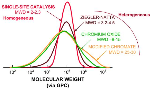
Fig. 2-25 Range MWD for polymers from gas phase process.
