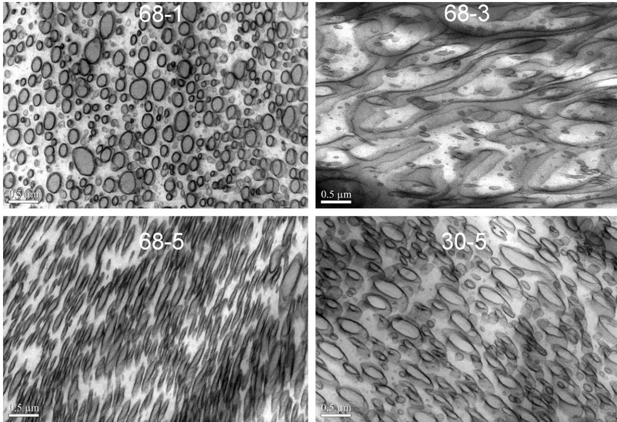
**Fig. 12-10** Transmission electron micrographs (TEMs) of immiscible polyethylene – Styrene polymer blends of varying chemistries. Courtesy of Barbara Wood and I-Hwa Lee, DuPont. Further examples of TEMs of immiscible blends can be found in Wood [35, 36].
