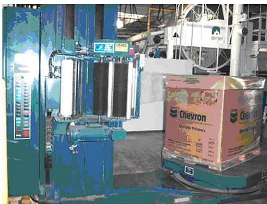
Fig. 15-9 Rotary pallet stretch cling wrapper.
