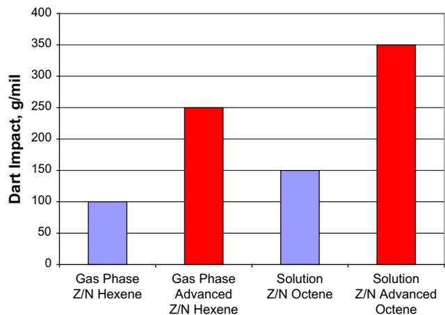
Fig. 2-34 Comparison of different Z–N catalyst systems in both gas phase and solution process on dart impact strength.
