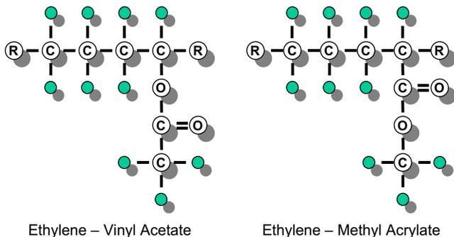
Fig. 2-19 Polar copolymers of ethylene EVA and EMA.
