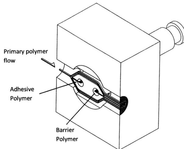
**Fig. 6-19** WELEX center layer block for introducing an adhesive/barrier/adhesive structure in the center of a flow stream, creating five layers from three flows. Principal flow from left to right and adhesive exits counter the primary flow to encapsulate the barrier flow (Courtesy Frank Nissel).
