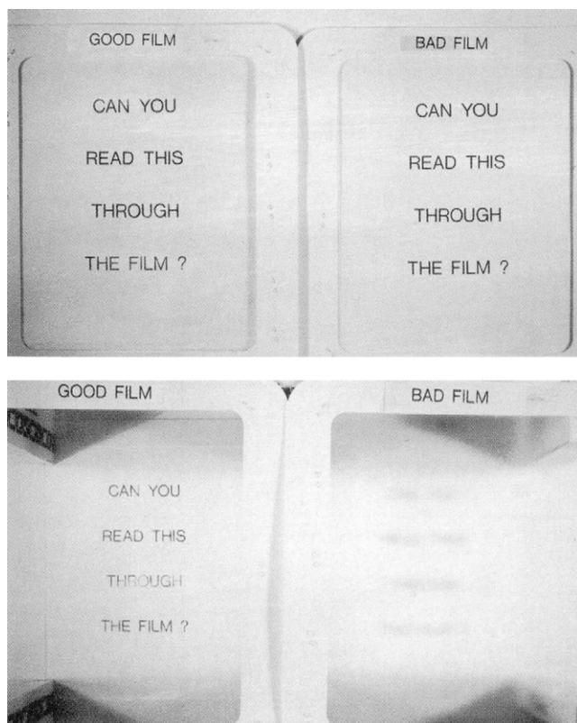
**Fig. 5-17** The effect of interfacial stability on contact clarity of coextruded films (top) versus see-through clarity (bottom).
