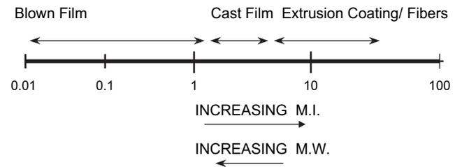
Fig. 2-4 Melt index of PE polymers used for various extrusion processes.
