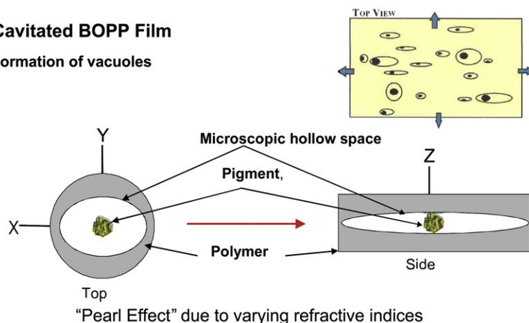
**Fig. 11-17** Cavitated BOPP film mechanism.
