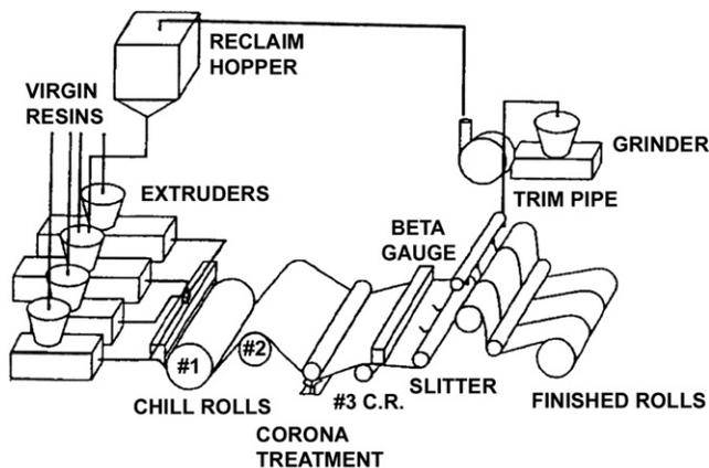
Fig. 9-5 Cast film process.
