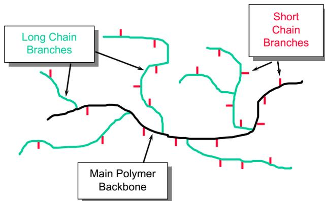
Fig. 2-16 LDPE homopolymer with LCB and SCB in the molecule.
