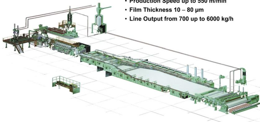
Fig. 11-6 A three-layer coextruded BOPP sequential stretching line.
