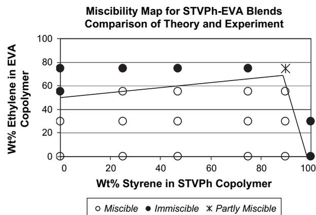
**Fig. 12-13** Example of using specific interactions between molecules to achieve miscible blends. Taken from Coleman et al [38].
