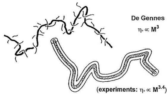
Fig. 5-12 Reptation model of polymer chain motion.
