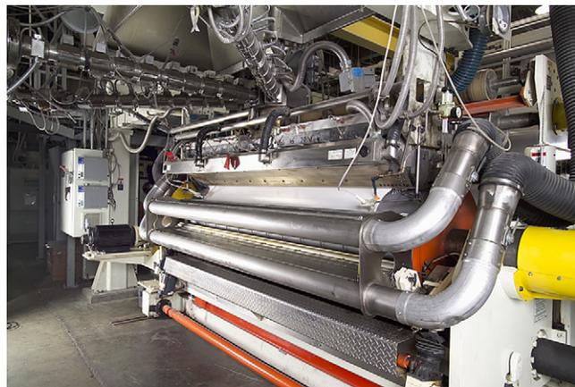
Fig. 9-7 Four melt pipes feeding multilayer die. Image provided by Davis-Standard <http://www.davis-standard.com/>.
