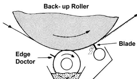
**Fig. 13-12** A blade coater against upwards moving web. From H. Weiss, *Coating and Laminating Machines*, Converting Technology Co., Milwaukee, 1977, with permission of Mrs Sheila Weiss.
