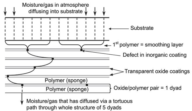
**Fig. 14-23** A schematic showing how a tortuous path improves barrier performance.
