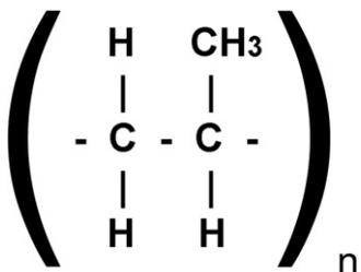
**Fig. 3-1** The polypropylene monomer unit. The subscript  $n$  indicates that this is a repeating unit that is connected to  $n$  other monomeric units.
