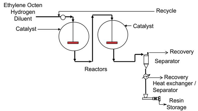
Fig. 2-26 Solution process (simplified).
