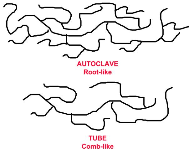
Fig. 2-17 Branching for autoclave and tube LDPE polymers.
