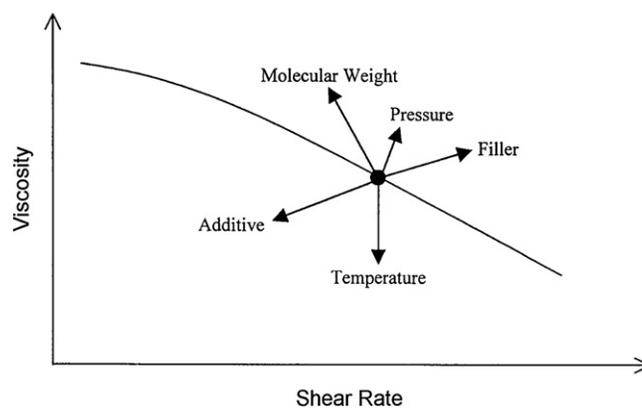
Fig. 5-7 The influence of various parameters on polymer viscosity.
