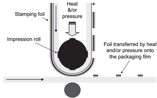
**Fig. 14-1** Schematic of hot or cold stamping foil: transfer process.
