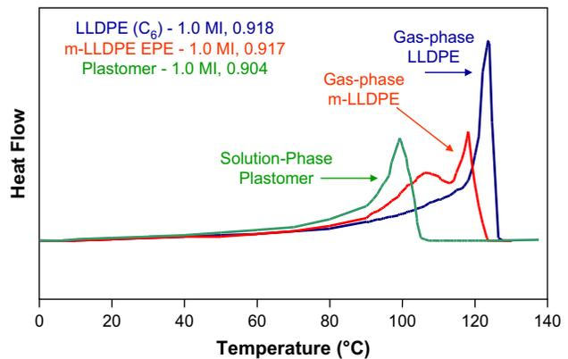
**Fig. 2-47** DSC curves for a SSC plastomer, an EPE m-LLDPE and an LLDPE (C<sub>6</sub>).
