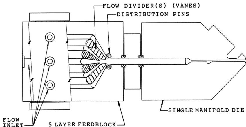
**Fig. 6-7** Cloeren five-layer adjustable vane feedblock (courtesy of Cloeren, Inc.).
