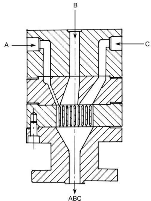
**Fig. 6-5** Three-layer Dow feedblock showing segmented flow plates.
