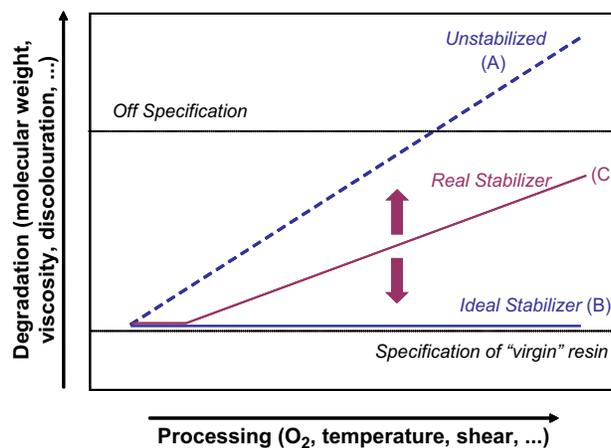
**Fig. 4-4** Principle of the utilization of antioxidants (and other stabilizers) during processing or conversion.
