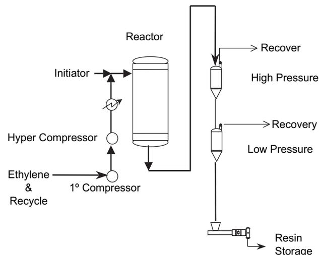
**Fig. 2-14** Autoclave reactor (simplified).
