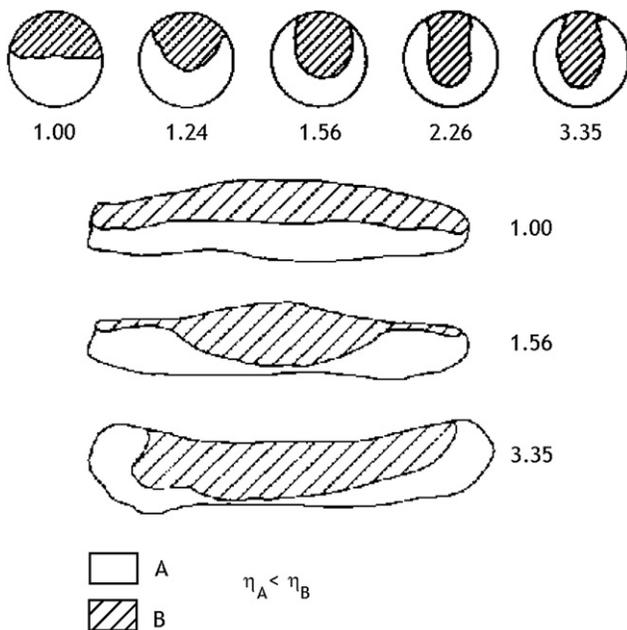
Fig. 5-15 Layer-to-layer flow rearrangement as a function of time.
