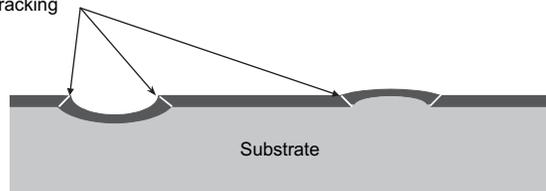
**Fig. 14-20** A schematic of how bumps and dents lead to stress raisers and subsequent cracking of the coating.
