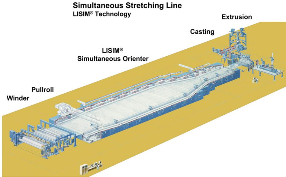
Fig. 11-12 Simultaneous stretching line.
