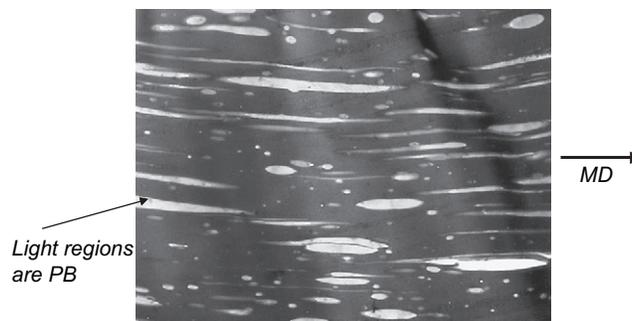
**Fig. 12-25** Elongated second phase (PB-1 in a polyolefin matrix) found in blown film. Photograph courtesy of DuPont.
