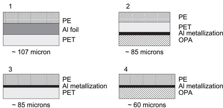
**Fig. 14-27** A schematic of the progression, (a-d), from the original foil packaging for coffee to the triple layer replacement and then to the double layer and then the thinner double layer current product.
