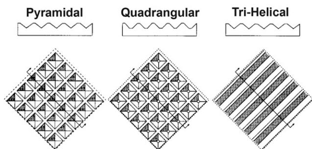
**Fig. 13-15** Gravure cell patterns. From *Modern Coating and Drying Technology*, (Cohen, E.D., Guttoff, E.B., eds), Copyright © 1992 Wiley-VCH. Reprinted with permission of John Wiley & Sons, Inc.
