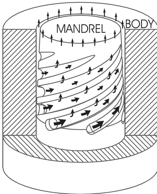
**Fig. 7-3** Conventional cylindrical spiral mandrel distribution system.
