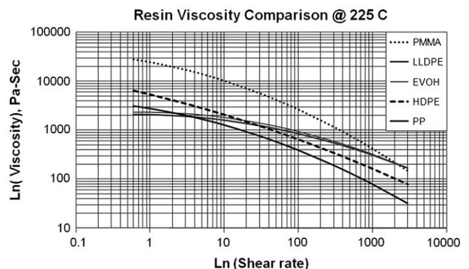
Fig. 6-10 Comparison of flow behavior of several resin types.
