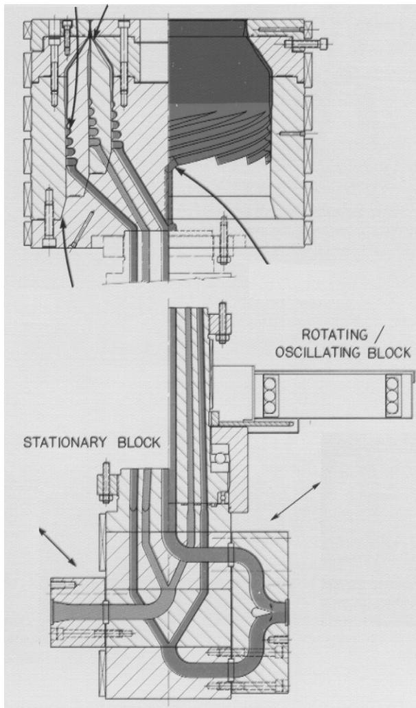
**Fig. 7-1** Conventional spiral mandrel type coextrusion die with rotating block.
