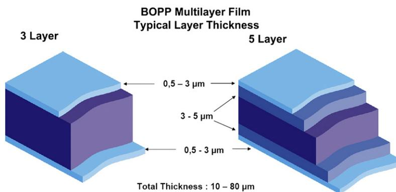
Fig. 16-6 Typical layer thickness of BOPP multilayer film.
