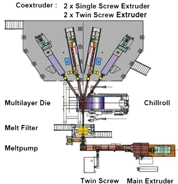
Fig. 16-3 A five-layer extruder configuration.
