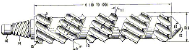
**Fig. 12-6** Saxton [23] mixing section.
