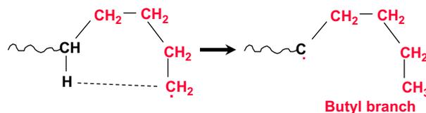
**Fig. 2-13** Mechanism for insertion of SCB in free radical polymerization.
