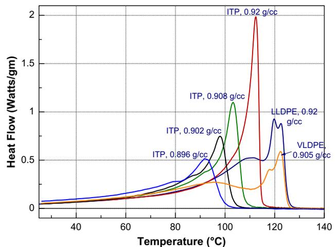
**Fig. 2-40** DSC curves comparing Z-N LLDPE and SSC octene copolymers (ITP).
