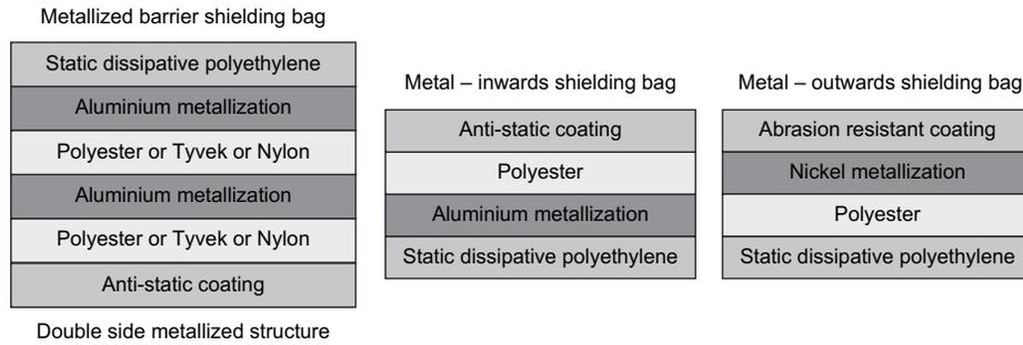
Fig. 14-10 Some of the basic metallized antistatic structures.
