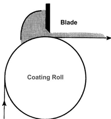
**Fig. 13-11** Rigid blade coater. From *Modern Coating and Drying Technology*, (Cohen, E.D., Guttoff, E.B., eds), Copyright © 1992 Wiley-VCH. Reprinted with permission of John Wiley & Sons, Inc.
