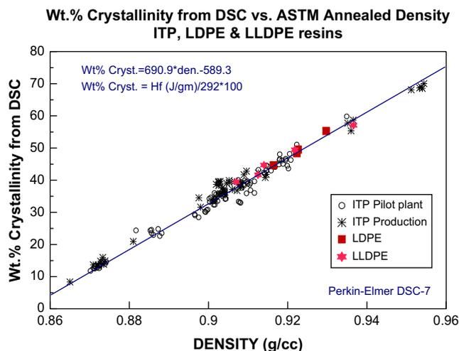
Fig. 2-18 Density versus crystallinity for PE polymers.
