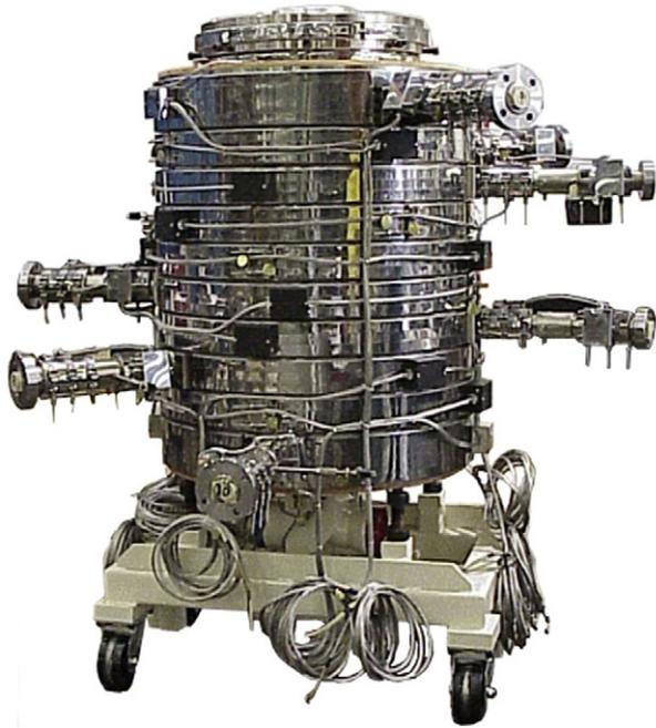
**Fig. 7-9** Photo of Brampton Engineering 10-layer stacked die.
