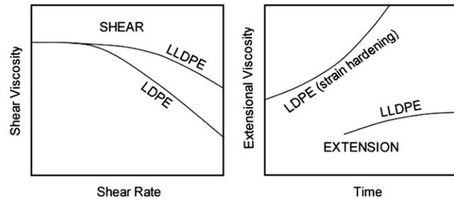
Fig. 5-9 Schematic representation of LDPE and LLDPE behavior in shear and extension.
