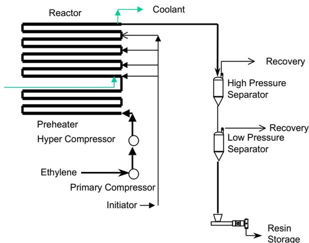
Fig. 2-15 Tube reactor (simplified).
