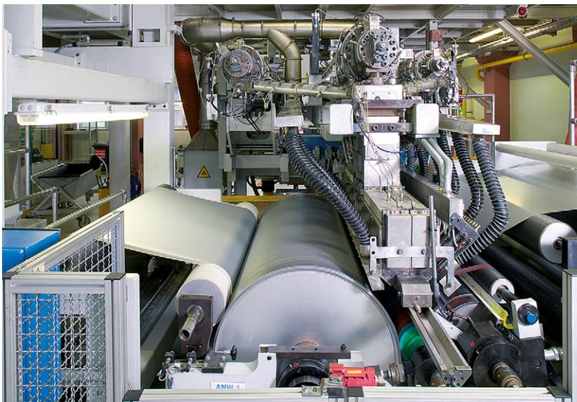
**Fig. 9-12** Multilayer extrusion coating station in operation. Image provided by Davis-Standard <http://www.davis-standard.com/>.
