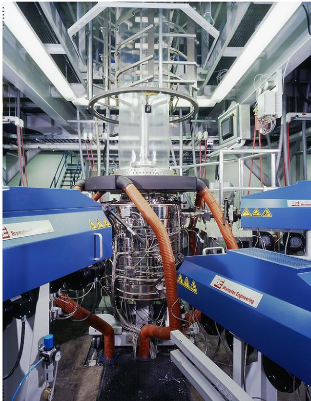
**Fig. 9-3** Nine-layer blown film die and bubble. Image provided by BE (Brampton Engineering) [www.be-ca.com](http://www.be-ca.com).
