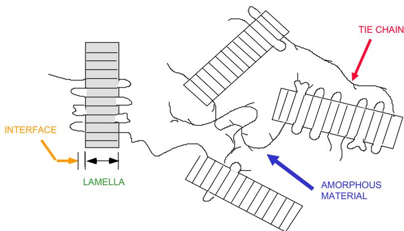
Fig. 2-42 Crystalline and amorphous regions of polyethylene.
