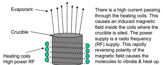
Fig. 14-13 A schematic of an induction heated evaporation source.
