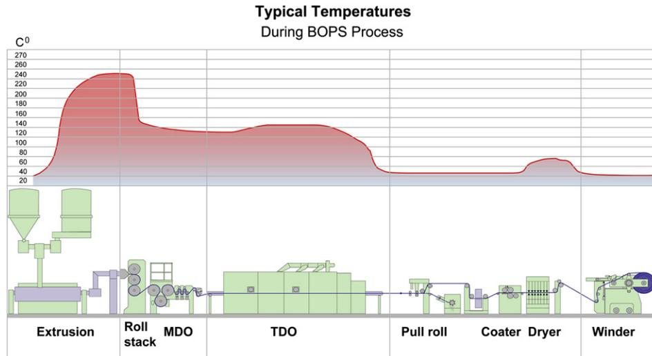
Fig. 11-30 Typical BOPS process temperatures.
