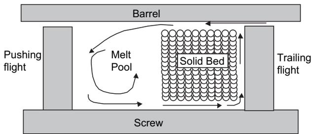
**Fig. 12-23** Single-screw extrusion solid bed melting model. Melting above and below the solid bed causes the minor component to form thin layers or striations in a 2-component polymer blend (after Lindt and Gosh [82]).
