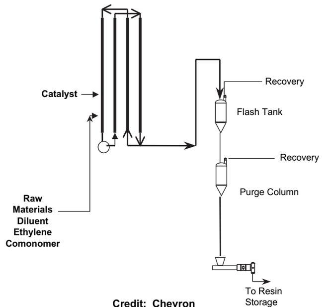
Fig. 2-27 Slurry loop process (simplified).
