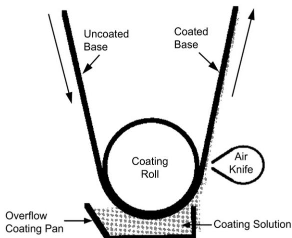
**Fig. 13-9** Air knife coater. From *Modern Coating and Drying Technology*, (Cohen, E.D., Gutoff, E.B., eds), Copyright © 1992 Wiley-VCH. Reprinted with permission of John Wiley & Sons, Inc.
