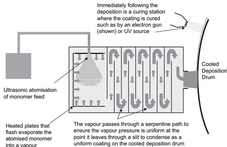
**Fig. 14-21** A schematic of in-vacuum polymer deposition.
