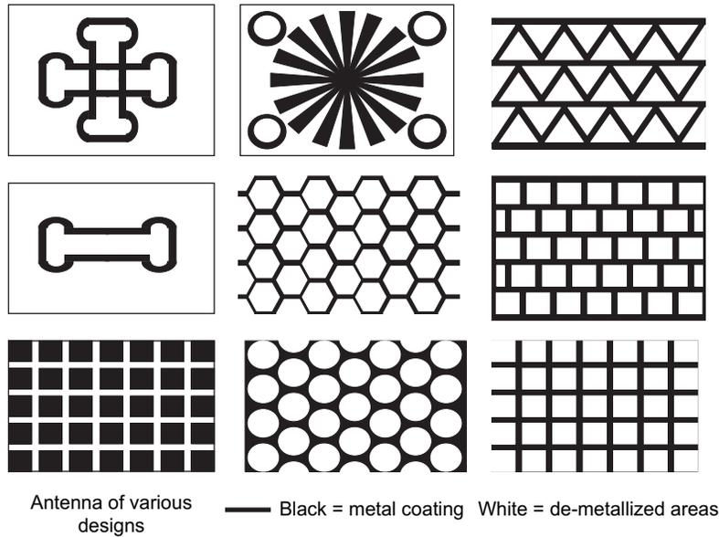
**Fig. 14-26** A schematic of various antenna shapes for microwave applications that could be produced by the oil printing pattern metallization technique.
