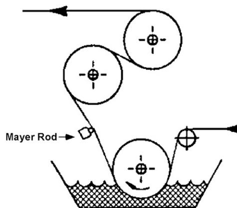
**Fig. 13-8** Mayer rod or wire-wound rod coater. From *Modern Coating and Drying Technology*, (Cohen, E.D., Guttoff, E.B., eds), Copyright © 1992 Wiley-VCH. Reprinted with permission of John Wiley & Sons, Inc.
