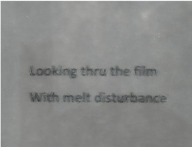
**Fig. 6-28** Looking through a film containing melt disturbance and held approximately 8 inches in from of the lettering, showing the image distortion caused by the variable film thickness from the melt disturbance.
