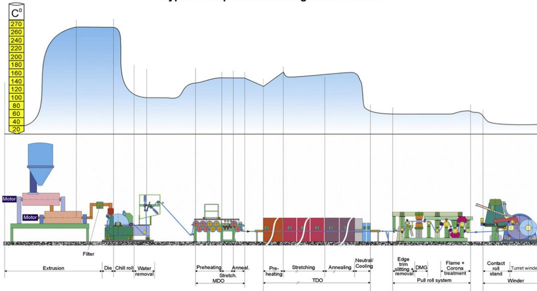
Fig. 11-7 Typical temperatures during the BOPP process.
