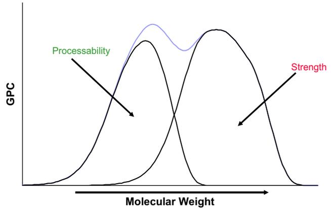
**Fig. 2-45** Enhanced molecular design using MWD.
