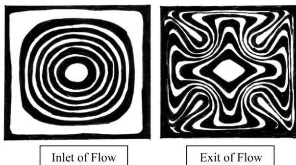
**Fig. 6-26** Secondary flow impact on layer rearrangement in square melt pipe flow (redrawn Fig. 5-33, from Dooley PhD Thesis, University of Eindhoven, 2002).
