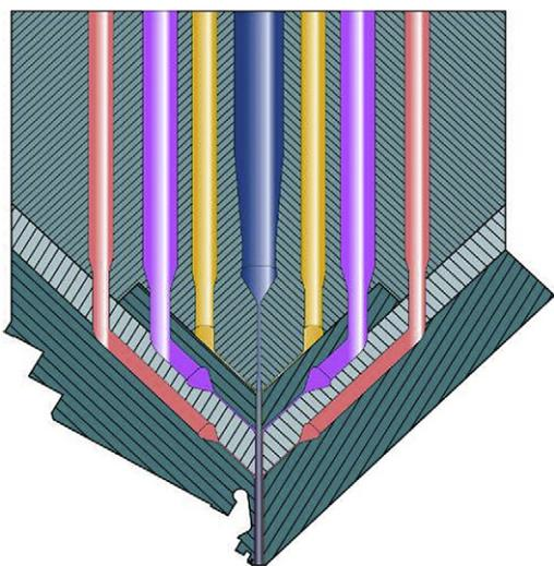
Fig. 16-5 Seven-layer coextrusion die.
