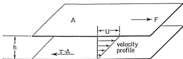
Fig. 5-1 Simple shear flow.
