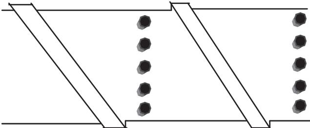
**Fig. 12-5** Pin mixing section.
