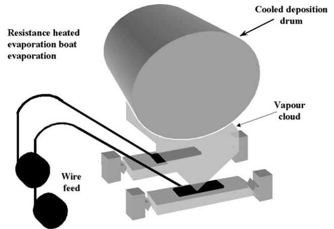
Fig. 14-12 Resistance heated boats in an aluminum vacuum metallizer system.
