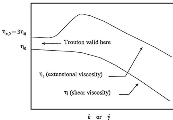
Fig. 5-8 Extensional and shear viscosity as a function of stretch and shear rate, respectively.
