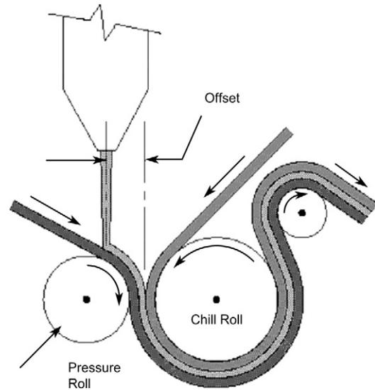
**Fig. 9-9** Extrusion lamination detail.
