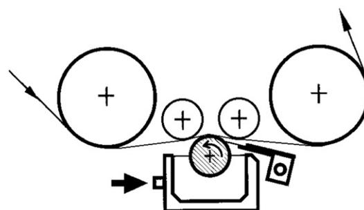
**Fig. 13-16** Microgravure™ coater. Reprinted with permission of Yasui-Seiki Co.
