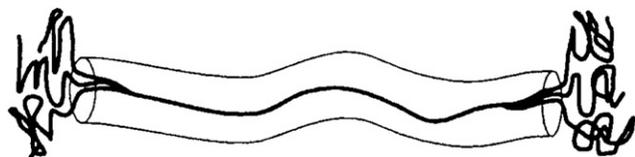
Fig. 5-13 The Pom-Pom polymer model.
