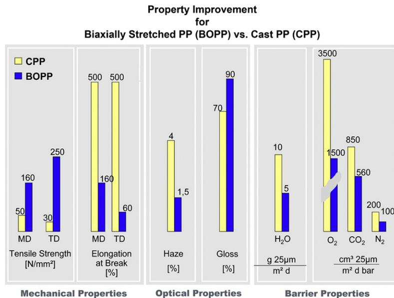
Fig. 11-2 Property improvement for biaxially stretched PP (BOPP) versus cast PP (CPP).
