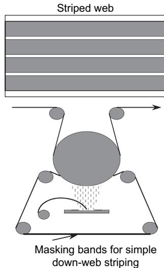
**Fig. 14-24** A schematic showing the process of using a masking band that produces simple stripes.
