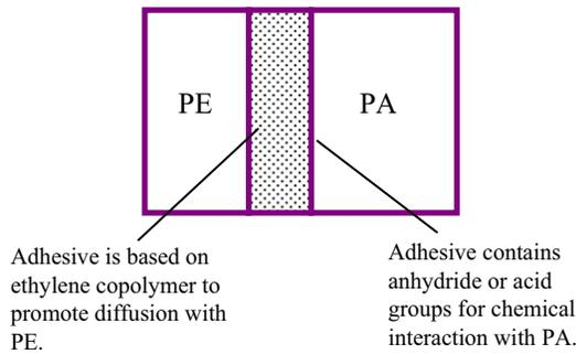
**Fig. 15-4** Coextrusion adhesive technology.
