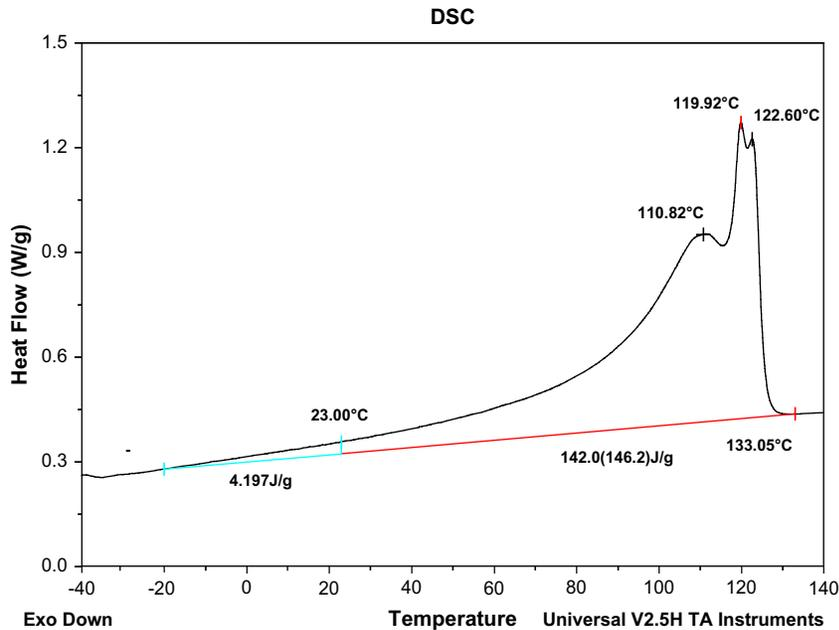
Fig. 2-32 DSC for LLDPE solution process octene heterogeneous copolymer.
