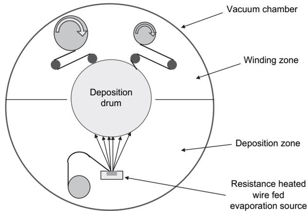
Fig. 14-11 Basic aluminum vacuum metallizer system.
