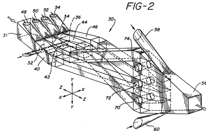
**Fig. 6-25** Fig. 2 of US Patent 2,269,995 showing square cross-section flow channels used for flow dividing and stacking to produce multilayer flows.
