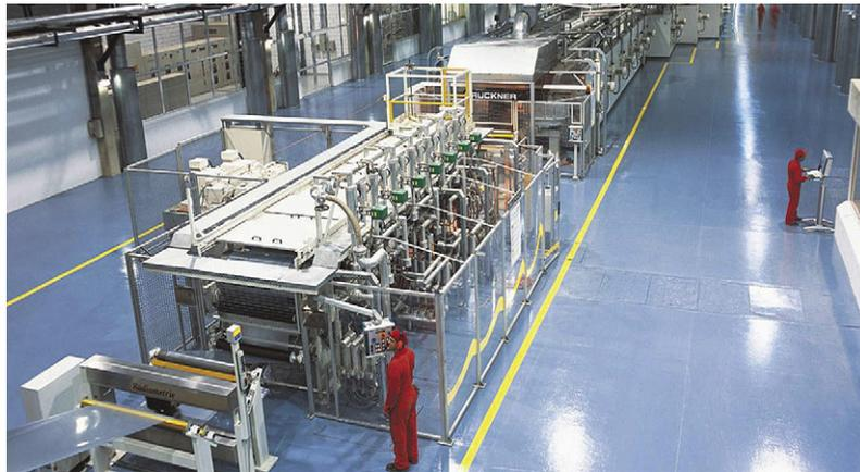
Fig. 11-8 Machine direction orienter with entrance.
