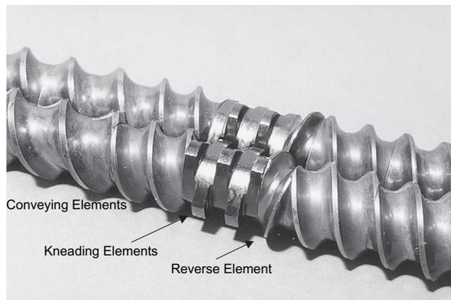
Fig. 12-9 Twin-screw extruder modular elements.
