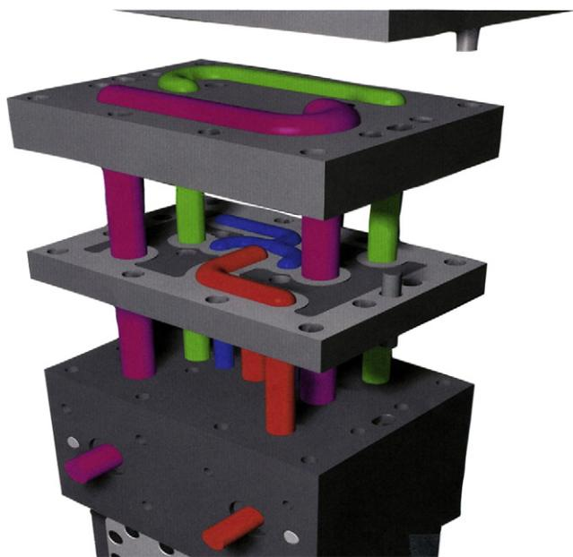
**Fig. 6-4** Segmented adapter with removable programming plates for re-routing of melt flow from the adapter to the feedblock.
