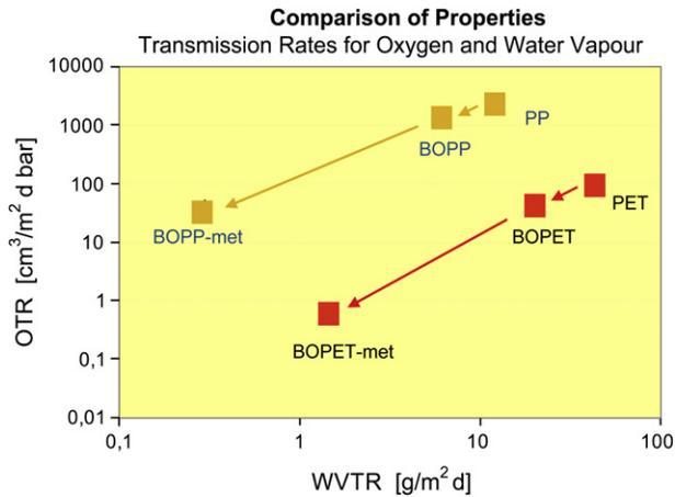
Fig. 11-23 Comparison of transmission rates for PP and PET.
