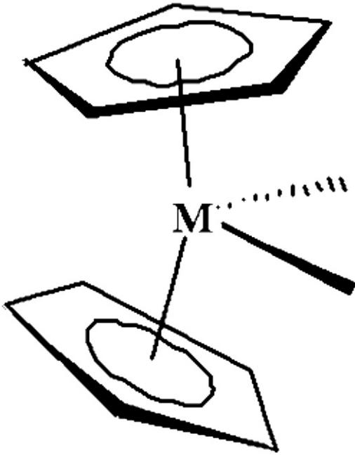
**Fig. 2-37** Metallocene catalyst typically contains a metal atom (zirconium) stabilized with, in this case, two cyclopentadienyl rings.
