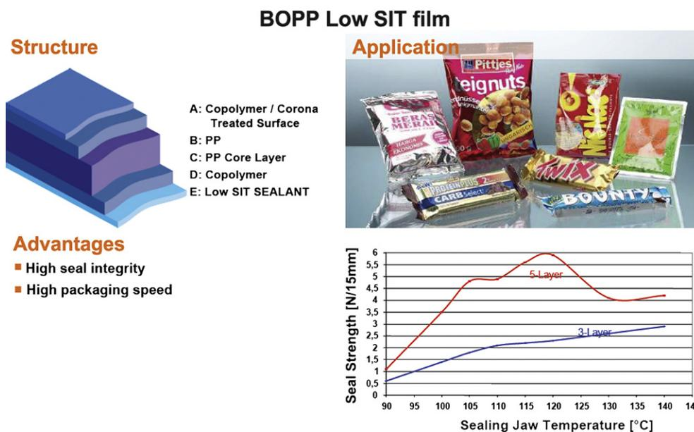
Fig. 16-7 Five-layer low seal initiation temperature (SIT) BOPP film structure advantages, applications and seal strength.
