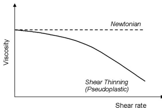
Fig. 5-2 Newtonian and shear-thinning viscosity behavior.
