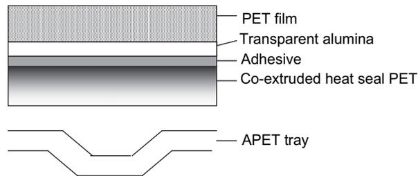
**Fig. 14-29** PET heat-seal laminate barrier-lidding material.
