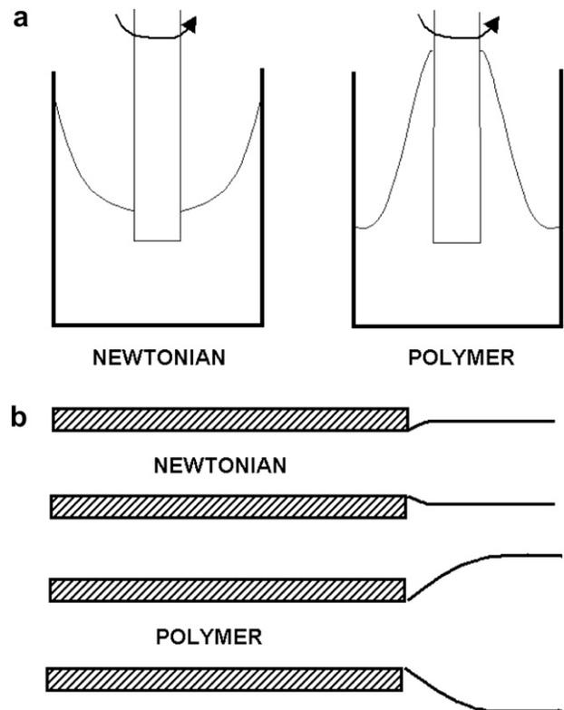
**Fig. 5-10** (a) Rod climbing (Weissenberg) effect in polymeric fluids; (b) extrudate swell.
