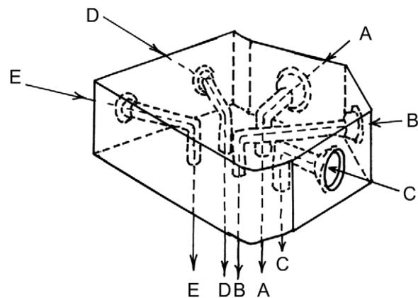
**Fig. 6-2** Fixed geometry adapter showing inflow from extruders A, B, C, D and E and the outflow of each extruder to the feed block. The adapter flow locations cannot be changed without replacing the adapter.
