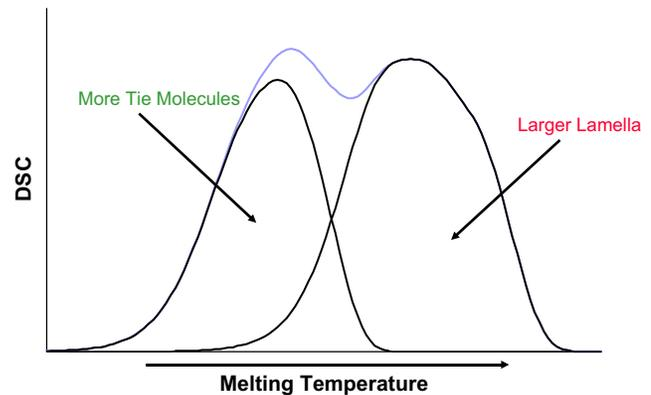
**Fig. 2-46** Enhanced molecule design using CD.
