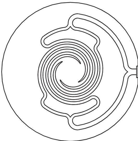
**Fig. 7-7** A flat spiral type of distribution system with four spirals.
