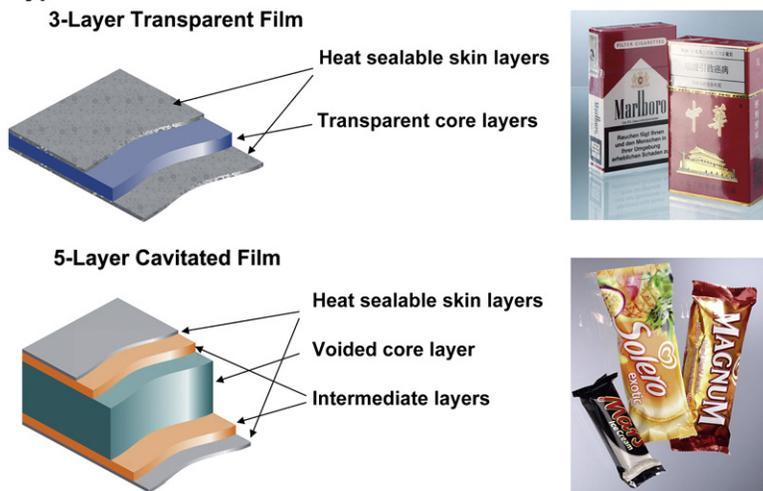
Fig. 11-16 Typical BOPP film structures.
