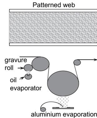
**Fig. 14-25** A schematic showing the much more versatile oil printing process for the production of finer and more detailed patterns.
