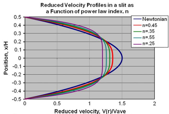
**Fig. 6-17** Plot of reduced velocity profiles for flow in a slit as a function of the power law index,  $n$  showing the blunt flow (plug flow) front increasing as  $n$  decreases.
