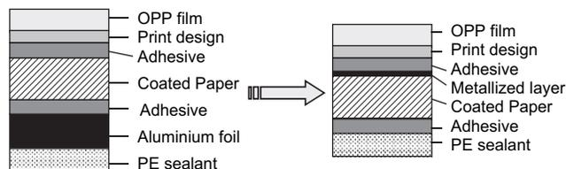
**Fig. 14-28** A schematic of an aluminum foil/paper label with a replacement label that uses a metallized polymer that replaces the paper and foil [43].
