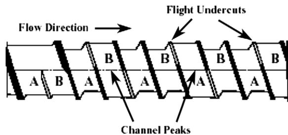
**Fig. 12-8** Illustration of a variable barrier energy transfer screw. Adapted from Hogan et al [26]. Courtesy of the Society of Plastic Engineers.
