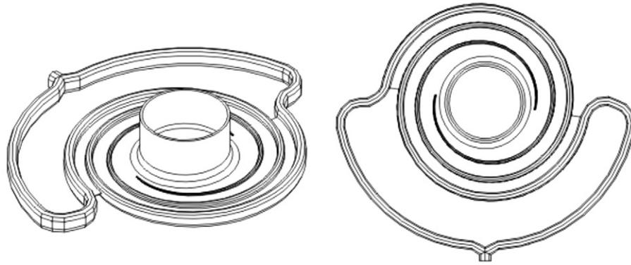
**Fig. 7-6** A flat spiral distribution system with two spirals.
