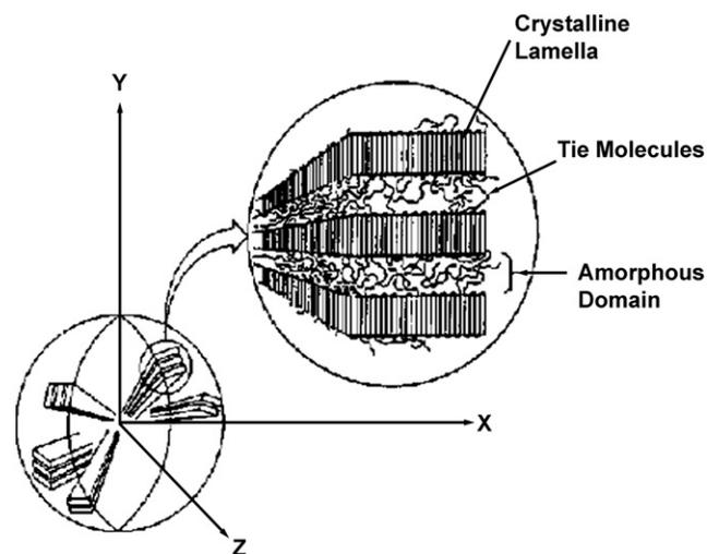
**Fig. 3-4** Spherulite crystal morphology showing the lamella, tie molecules and amorphous domain.
