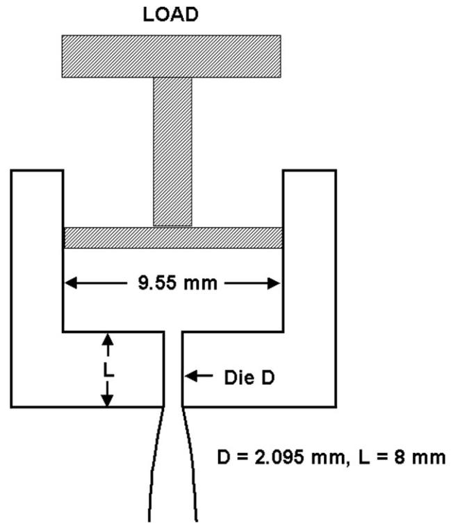
Fig. 5-4 Schematic of a melt indexer.
