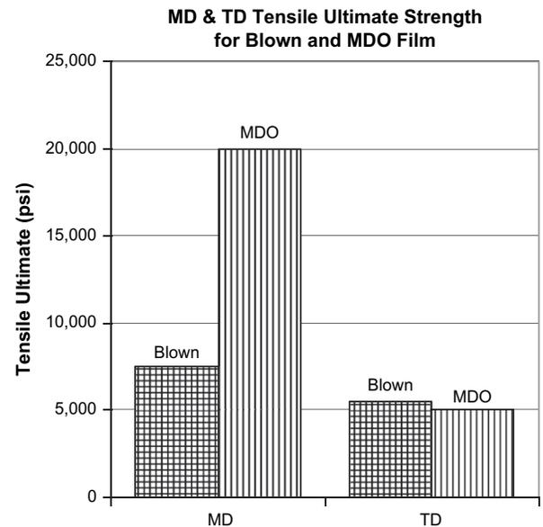
Fig. 10-9 MD and TD tensile ultimate strength for blown and MD oriented LLDPE [3].
